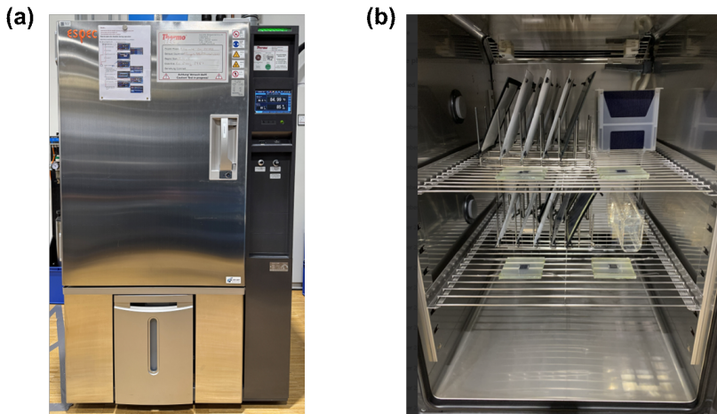
Figure 3.10: (a) Appearance of the climate chamber, and (b) solar module samples in the climate chamber.
