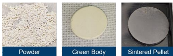
Figure 4-1: Sample stages of electrolyte supported button cells (d = 25 mm).
