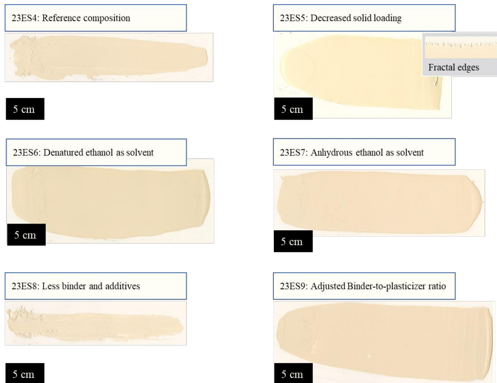
Figure 5-7: Impact of differently adapted slurry compositions on casting results. Manually cast slurries, scanned, color saturation digitally changed to enhance defect visibility.
