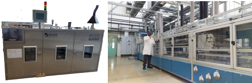
Figure 3-4: left) Medium size tape caster, “KaroCast”, KMS, right) industrial-size tape caster “JuCast”, KMS.
