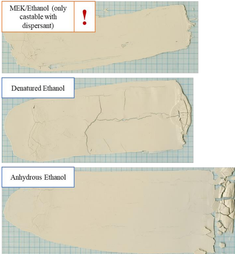
Figure 5-5: Impact of solvent on casting results for slurries composed only of ceramic powder, solvent, and binder without plasticizers (manually cast slurries, scanned).
