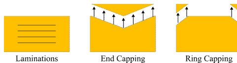
Figure 2-10: Pressing defects, formation of layers, end capping and ring capping after Reed. [61]
