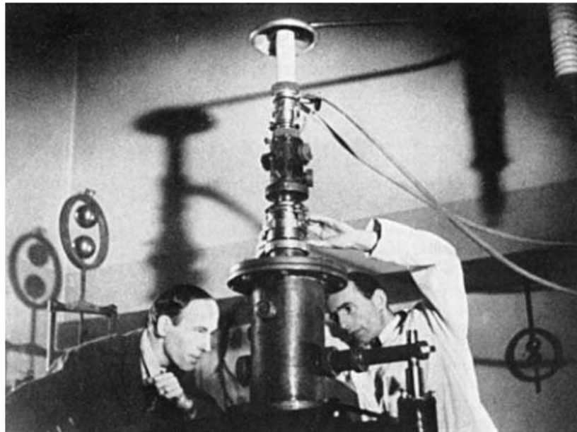
Figure 1.5: The first prototype electron microscope, built by Ernst Ruska and Max Knoll in 1931 at the Technical University of Berlin. The instrument employed two magnetic lenses in series to form an “electron-optical” imaging system, demonstrating the foundational principle of electron microscopy. Although its resolution was initially comparable to that of a light microscope, this device paved the way for later designs that exceeded optical limits. Adapted from Williams et al. [19].
