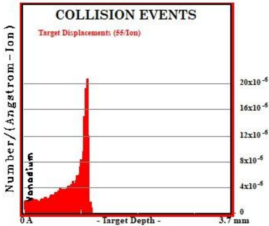
Figure 2.2 Representative SRIM/TRIM collision-events output from the vanadium simulation package. Collision-event data are used for post-processing damage-rate calculations
