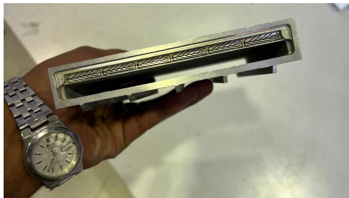
Figure 3.1 Machined target/cooling-channel component documented during the facility visit. The channelled geometry illustrates the importance of thermal management in target design.
