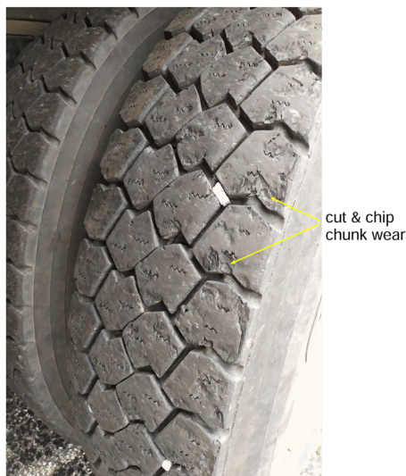
FIG. 26. Cut and chip wear of truck tires results from removing macroscopic ( \sim \text{cm} ) patches of rubber from the tire surface when driving on very rough road surfaces with long wavelength or large scale ( \sim \text{cm} ) inhomogeneities such as gravel or roots (R. Stoczek, private communication).
