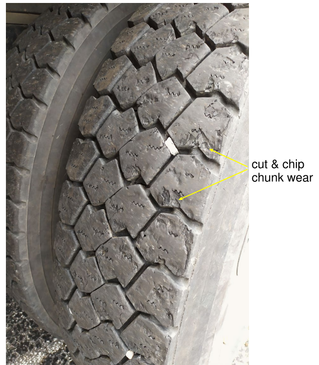
Fig. 21 Cut-and-chip wear on a truck tire due to macroscopic ( \sim \text{cm} ) rubber fragment removal when driving over very rough surfaces such as gravel or embedded roots. Adapted from [11]
