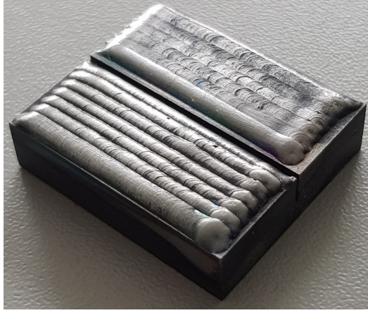
Figure 6.4: LMD-w single layers were deposited on the top surfaces of this tungsten double tile. On the left half one normal layer and on the right one smoothed layer was deposited, using the process parameters listed in table 6.3 [171].
