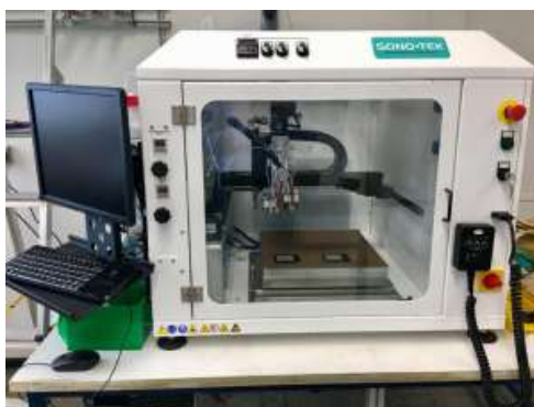
Figure 4.3. Photographic image of the ultrasonic spray-coating device (Exactacoat, Sono-Tek) used for electrode fabrication.
