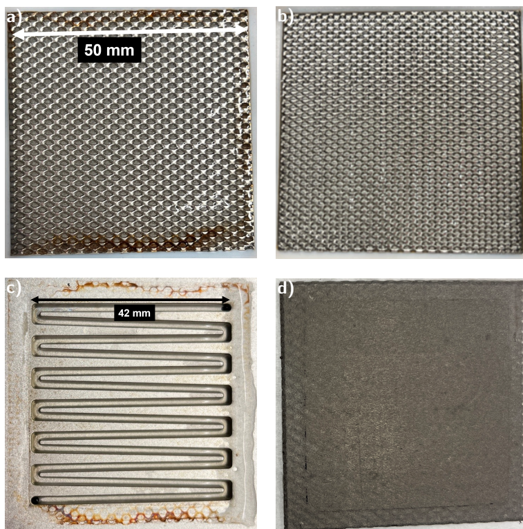
Figure 7.14. Photographs of a) FF-facing side of SMF8_Ti post mortem; b) FF-facing side of SMF8_Ti post mortem; c) Anode flowfield used in conjunction with SMF8_Ti post mortem; d) CL-facing side of SMF8_Ti post mortem.
