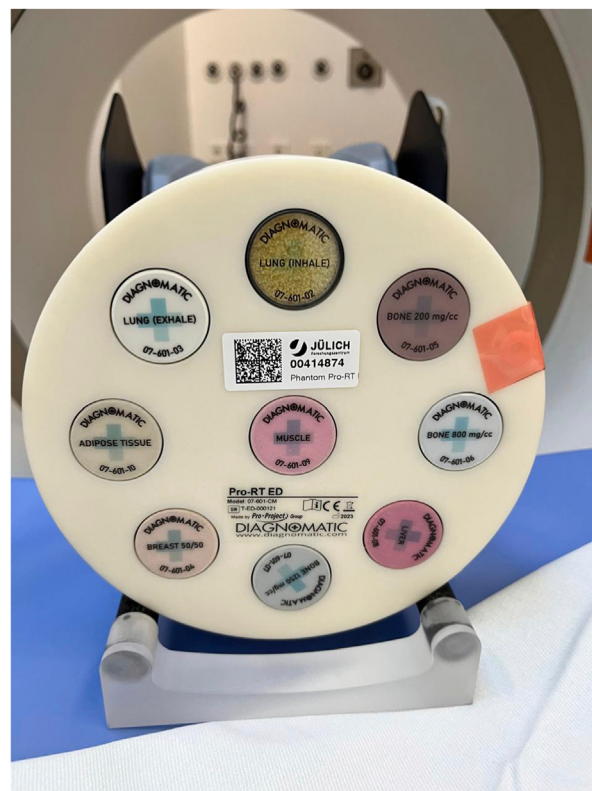
FIGURE 2 Insert layouts for the DIAGNOMATIC Pro-RT ED phantom. The inserts—arranged clockwise starting from the top—are lung (inhale), solid trabecular bone 200 mg/cc HA, solid dense bone 800 mg/cc HA, liver, solid dense bone 1250 mg/cc HA, breast, adipose, lung (exhale), and muscle.
