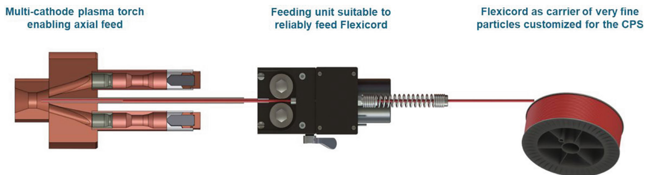
Fig. 33 Schematic view of the set-up for CPS (Cord Plasma Spray) process.
