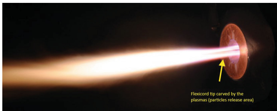
Fig. 36 View of the CPS in operation revealing the tip of the flexicord carved at the exit of the nozzle, indicating the location where the particles are released into the plasma stream
