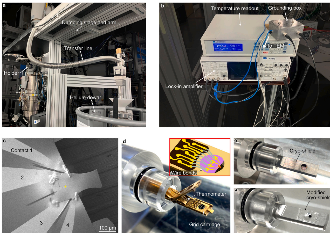
Fig. 1. Measurement setup overview. (a) Photograph of the helium dewar, helium transfer line inserted into the back of the TEM holder, and the arm of the damping stage that supports the helium transfer line. (b) Photograph of the temperature sensor readout, lock-in amplifier, and grounding box. A diagram of the electrical measurement setup is given in Fig. S2. In (a, b) the background has been blacked out to emphasize the equipment used in this work. (c) SEM image of NbN device 1. The numbering of the electrodes is indicated on the image. (d) TEM sample holder with opened tip. The grid cartridge with the TEM grid has been mounted onto the holder. The location of the thermometer is indicated. The TEM sample holder is placed on a holder stand. The inset shows a diagram of the TEM grid, the grid cartridge, and the wire bonds connecting both together. (e, f) Photographs of the TEM sample holder with the tip closed and encased in the (e) regular and (f) modified cryo-shield.
