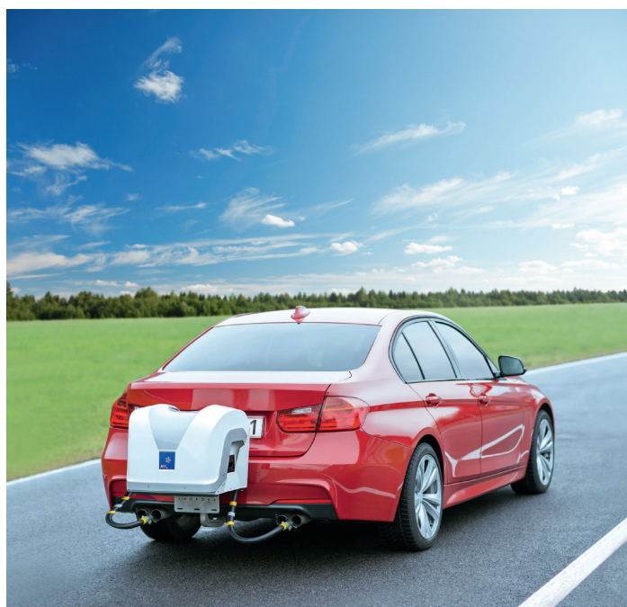
Fig. 5. A PN-PEMS based on the automotive Partector. Picture © AVL List GmbH.
