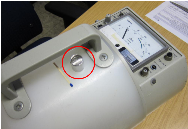
Fig. 3.1: AmBe neutron source used for detector calibration. The source's \alpha activity is 350 MBq, yielding a neutron production of 20000 n/s. The measured dose rate emitted by this source is about 10 \mu\text{Sv/h} .
