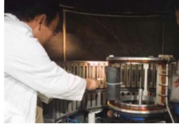
Fig. 8.5: (left) Magnetic field setting in a xyz-coil system for an adiabatic nutation of the polarization of cold neutrons in horizontal x-direction at the sample turning to a vertical (guide) field B_z at further distance from the sample. (right) A photo of the xyz-coil system in the DNS instrument at the FRM-2.
