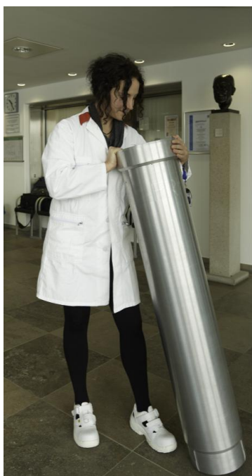
Fig. 3.5: A model of the fuel element of the FRM II research reactor. The inclined plates contain the fuel, the cooling water flows in between the fuel plates. The central channel is the position of the control rod. The core of FRM-2 is the most compact ^{235}\text{U} reactor core ever built. (Copyright W. Schürmann, TU Munich)
