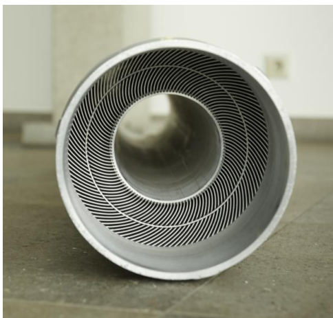
Fig. 3.5: A model of the fuel element of the FRM II research reactor. The inclined plates contain the fuel, the cooling water flows in between the fuel plates. The central channel is the position of the control rod. The core of FRM-2 is the most compact ^{235}\text{U} reactor core ever built. (Copyright W. Schürmann, TU Munich)
