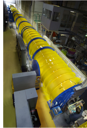
Fig. 15.5: Left: Scattering triangle for a small angle measurement. The ellipsoids represent the longitudinal and transverse uncertainties of initial and final wave vector \mathbf{k} and \mathbf{k}' . The longitudinal uncertainty corresponds to the wavelength resolution, the transverse to the angular collimation. Right: Detector tank of D11 at the ILL
