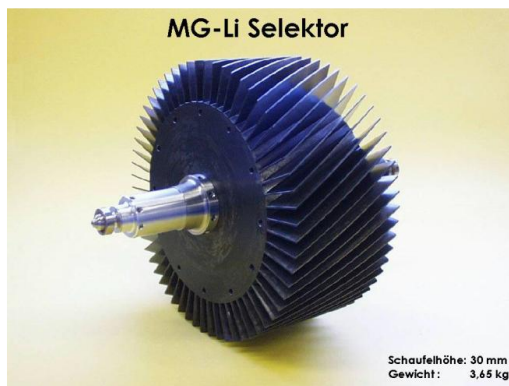
Fig. 3.10: Turbine wheel of the velocity selector used at KWS-3. The selector blades consist of a MgLi alloy with neutron absorbing ^6\text{Li} .
