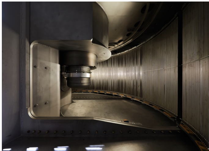
Fig. 15.12: Large area detector of the TOPAS spectrometer under construction at FRM II. The height of the detector tubes is 2.2 m, it has an active area of 15 m 2 and covers a solid angle of approximately 2 sr.
