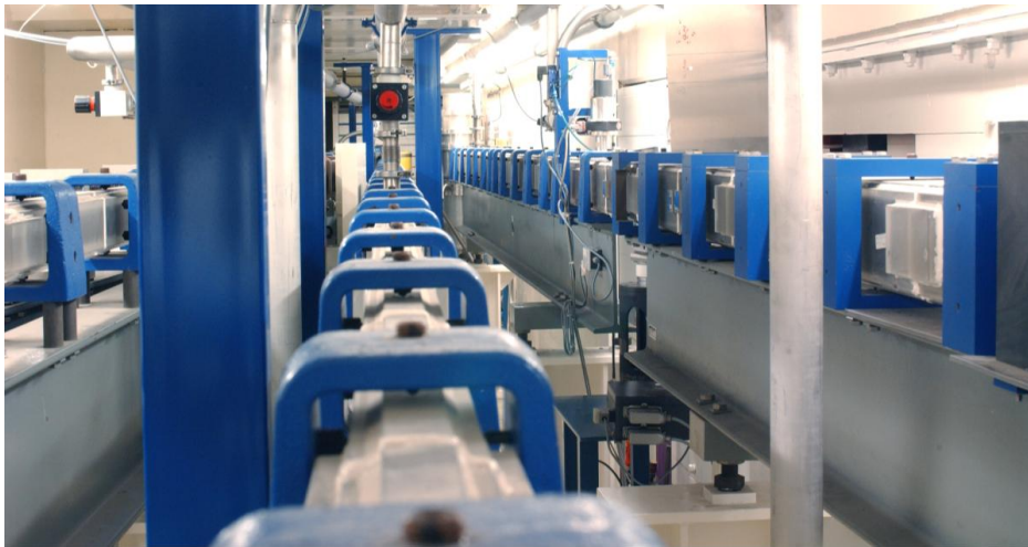
Fig. 3.12: Neutron guides serving the cold neutron instruments at the former FRJ-2 research reactor in Jülich.
