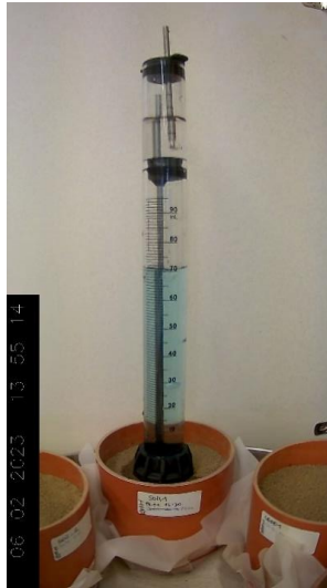
Fig. A.4. Mini-disk infiltrrometer (MDI, Meter Group AG, Munich, Germany) filled with blue colored water placed on a soil-filled PVC column (10 x 10 cm).
