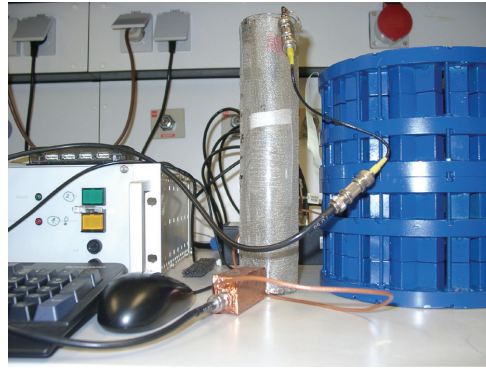
Fig.5.1.Halbach magnet of 0.15T together with RF coil and STELAR spectrometer
