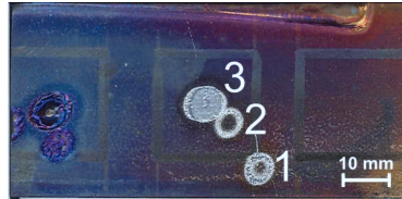
Figure 3.26: Surface of a steel plate used for aiming. The lines show the position of the tiles located below the plate. Melt traces of the first, second and third shot are clearly visible (numbers). After the last shot the plate was removed and the actual experiment was started. The plate was used in a test of the second mock up design (fig. 3.15) with r_{\text{circ}} = 3.8 mm. Although it became apparent that this radius is too large, the circles proved the working principle of the circular loading pattern (section 3.4).
