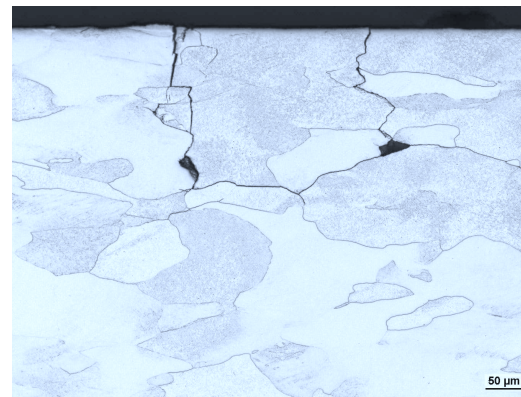
Figure 5.26: Cross section image of sample 091E5 loaded with 10^5 pulses of F_{\text{HF}} = 9 \text{ MWm}^{-2}\text{s}^{0.5} at T_{\text{surf}} \approx 200^\circ\text{C} . These conditions are the same as in figure 5.25, just at T_{\text{surf}} \approx 200^\circ\text{C} instead of T_{\text{surf}} \approx 700^\circ\text{C} .
