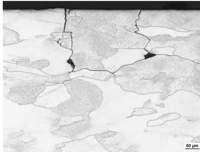
Figure 5.26: Cross section image of sample 091E5 loaded with 10^5 pulses of F_{HF} = 9 \text{ MWm}^{-2}\text{s}^{0.5} at T_{\text{surf}} \approx 200^\circ\text{C} . These conditions are the same as in figure 5.25, just at T_{\text{surf}} \approx 200^\circ\text{C} instead of T_{\text{surf}} \approx 700^\circ\text{C} .
