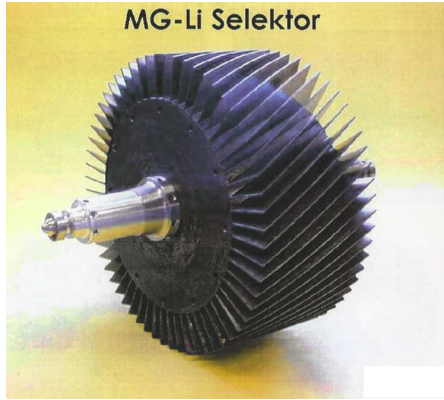
Fig. 2: The neutron velocity selector of the small angle scattering instrument KWS-3 at the research reactor Garching FRM-2. This selector was especially manufactured for larger wavelengths (above 7\text{\AA} ).
