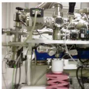
(e) Evaporation chamber, with the molecule reservoir below, cooled in a cup of iced water
