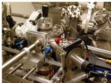
(b) Sputter chamber with the argon ion source with magnet, on the right
