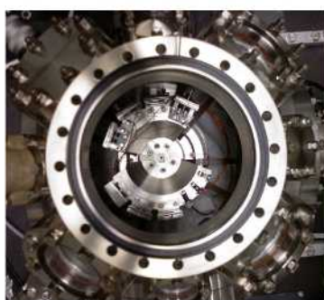
(d) Storage carousel inside the chamber, as seen through an open port during assembly
