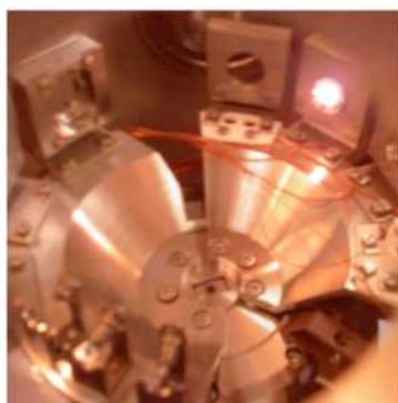
(f) Heating carrier in operation, mounted on the storage carousel in vacuum, emitting IR-radiation
