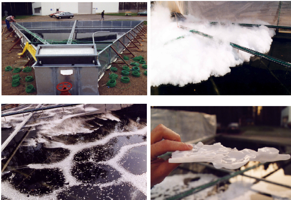
Figure 8-11. LN 2 release test facility KIWI at FZJ (top left) with a spreading pool (top right) and typical ice structure formation on the water surface (bottom) [Dienhart 1995]
