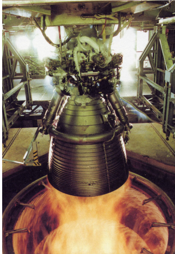
Figure 7-4. Testing of the Vulcain engine for the Ariane rocket (Courtesy of DLR)
