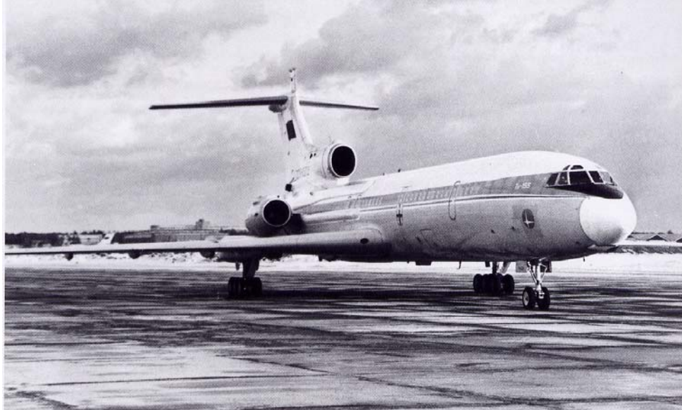
Figure 7-11. Tupolev 155 “Flying Laboratory” of 1988 with the central engine fueled by LH 2 or LNG (Courtesy of PSC Tupolev)
