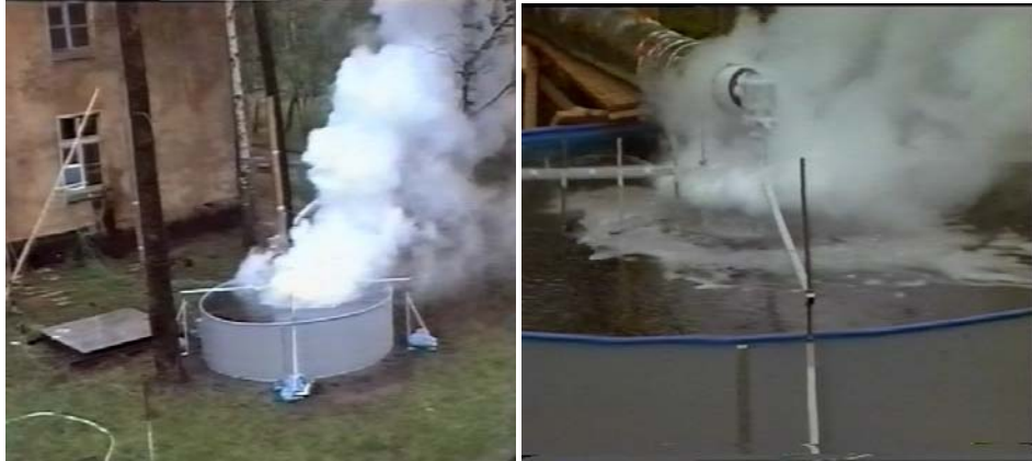
Figure 8-13. LH 2 pool spreading on water during BAM tests in 1996 with ice layer visible at test end (Courtesy of BAM)
