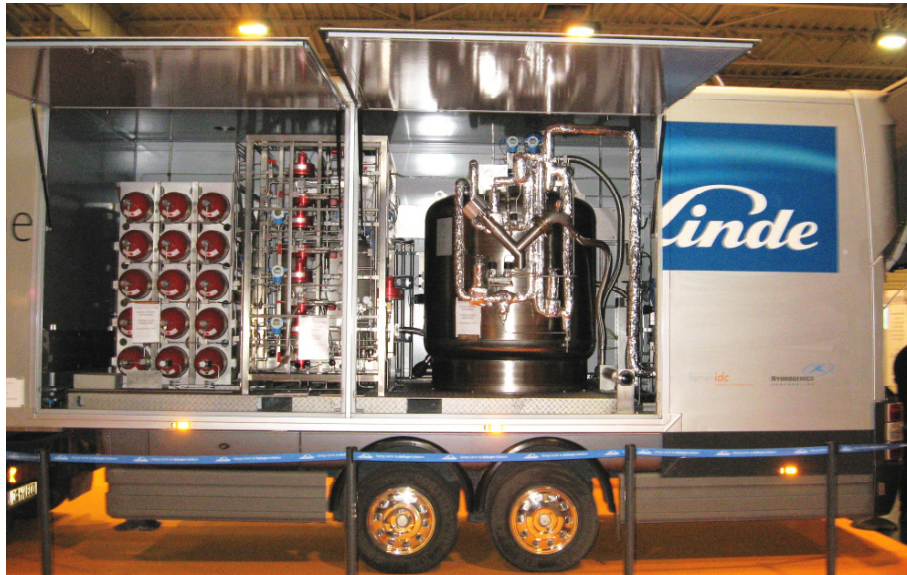
Figure 7-20. Linde trailer-mounted filling station for GH 2 and LH 2 fuel
