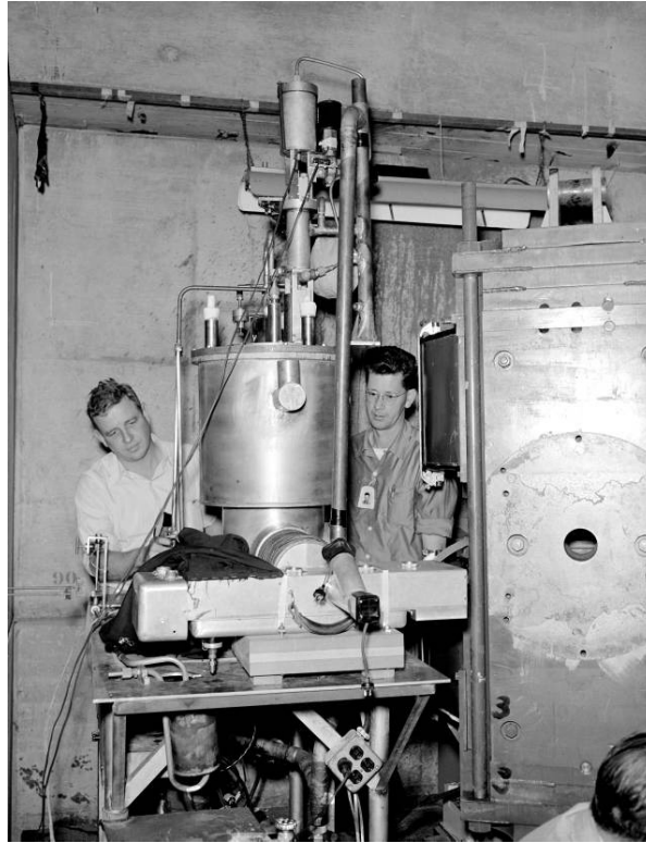
Figure 7-26. First LH 2 chamber by Alvarez (right) (Courtesy of Ernest Orlando Lawrence Berkeley National Laboratory)
