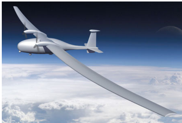
Figure 7-13. HALE, concept of an unmanned aircraft with a Ford internal combustion engine running on hydrogen (Courtesy of Boeing - Chuck Schroeder)
