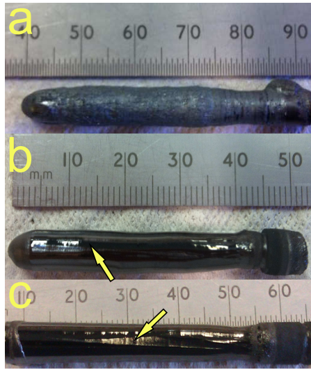
Figure 4.5: \text{YbFe}_2\text{O}_{4-\delta} Crystal Boules
