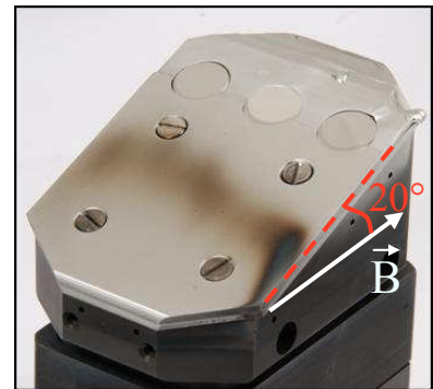
Figure 1. Test limiter with mirrors after exposure
