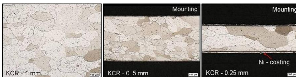
Figure 5.155: Optical micrographs showing cross sections of Crofer 22 APU (KCR) samples with different thicknesses after 2000 h oxidation at 800 °C in laboratory air. (Samples etched with 5% \text{H}_2\text{SO}_4 ).
