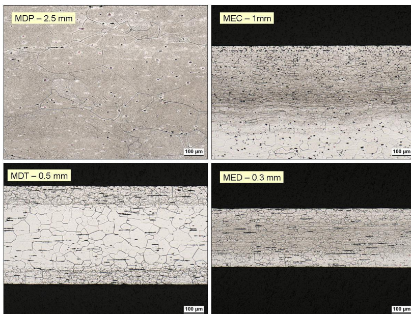
Figure 4.2: As received microstructures of investigated Crofer 22 H batches.
