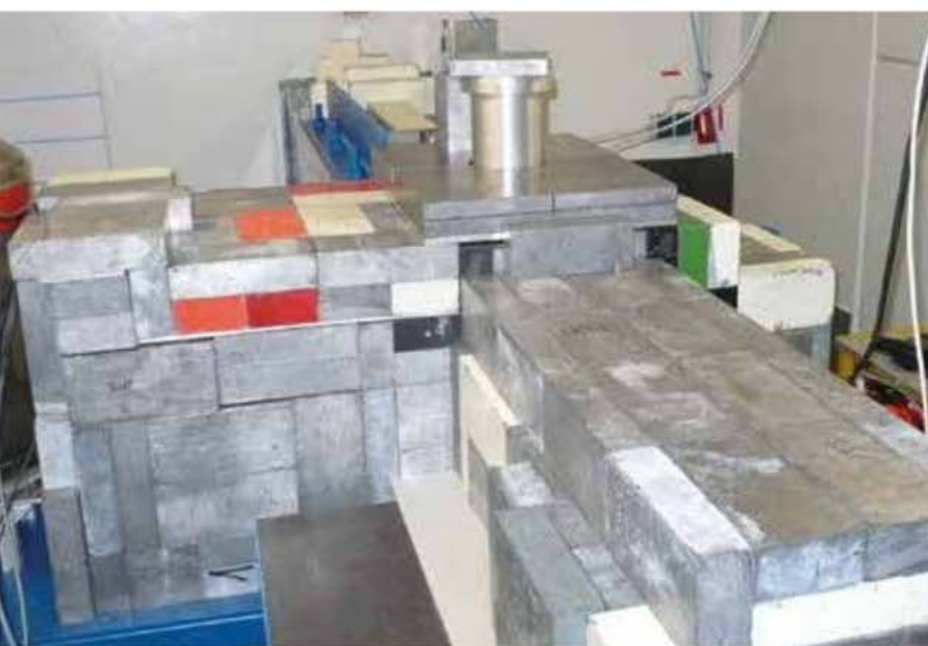
Figure 1: High-purity germanium detector with Compton-suppression system in an open lead shielding.
