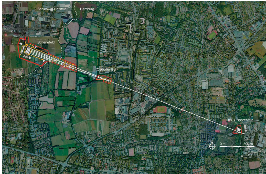
Fig. 3: Layout of the European XFEL, showing the trace of the underground tunnels running under the northwest districts of Hamburg and the neighbouring town of Schenefeld
