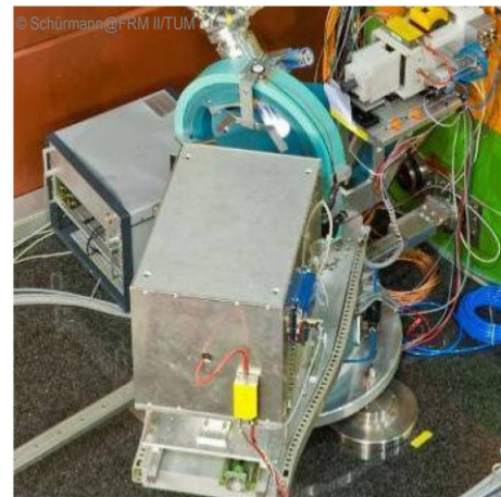
Fig. 16: Classical neutron diffractometer HEiDi with Eulerian cradle and mounted cryostat
