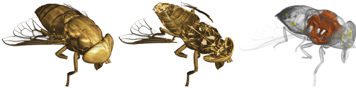
Fig. 19: Tomographic views onto a fly which was studied using cold neutrons with presently highest possible resolution (pixel size 13.5 \mu\text{m} ; sample size 12 mm); the advantage of the high contrast for hydrogen enables to see very much detail – better than naked human eye can do.
