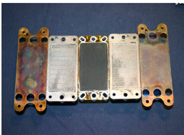
Figure 1: Single cell components after 3000 hrs of operation.
