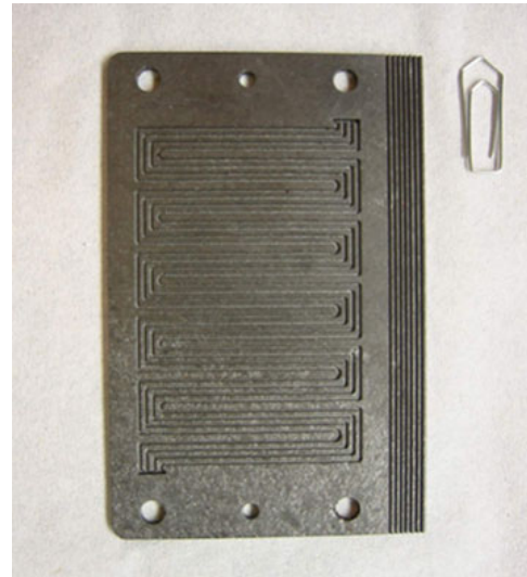
Figure 5: 27,6 cm 2 active area bipolar plate based with cooling fins.
