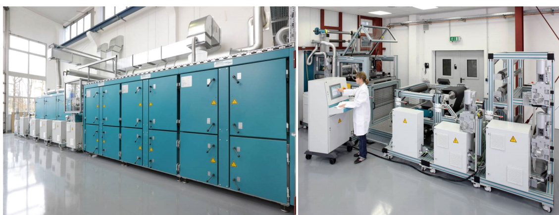
Figure 2: Flexible coating machine made up of several modules.
