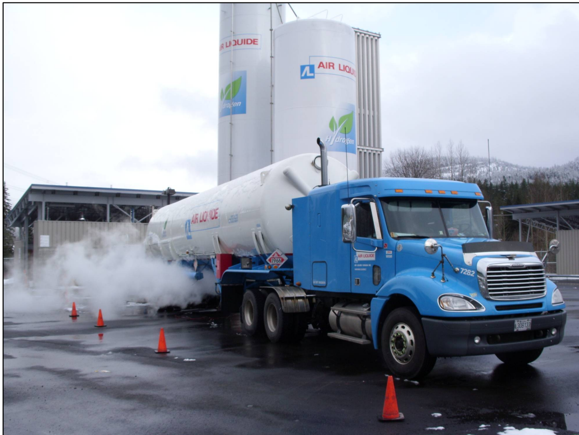
Figure 2: Liquid hydrogen delivery to Whistler refuelling station.
