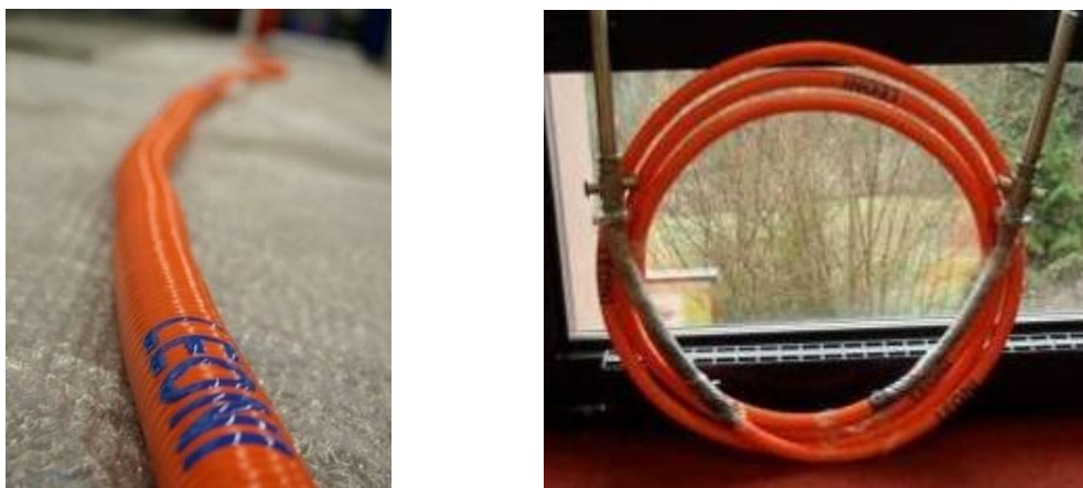
Figure 4: icefuel ® cable sample (outer diameter: ca. 40 mm; max. transport capacity: 100 – 200 kW LHV ; LEONI, Nuremberg).
