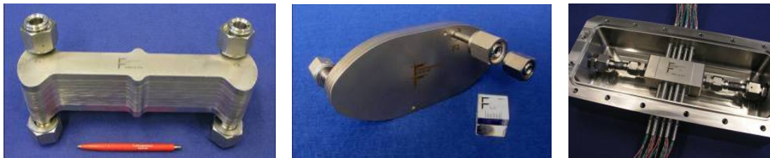
Figure 5: Various micro heat exchangers being developed for cooling, heating or other processing of hydrogen (IMVT, Karlsruhe).
