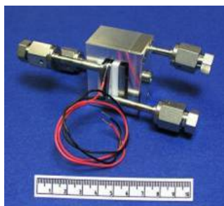
Figure 6: Lab scale micro heat exchanger equipped with a thermoelectric generator (DLR, Cologne and IMVT, Karlsruhe).
