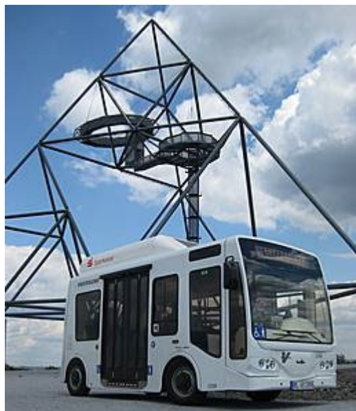
Figure 4: Fuel cell midibus in the project HYCHAIN-MINI TRANS.
