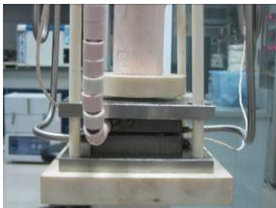
Figure 3: The assembled SOEC stack with three cells.
