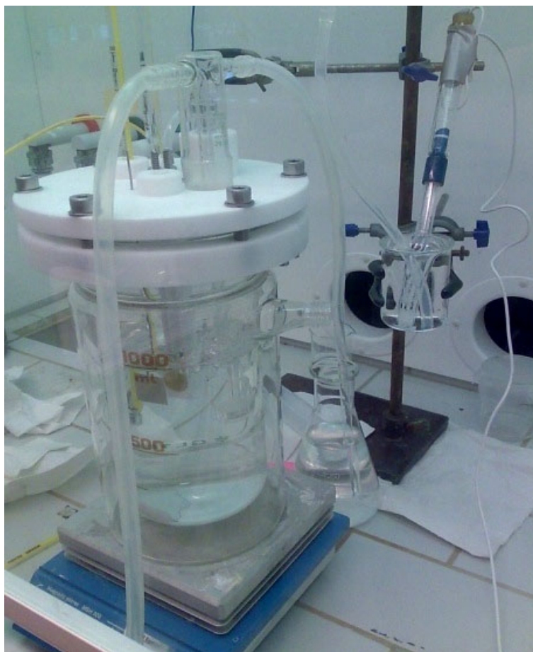
Figure 1: Three-electrode cell used in LSV test.
