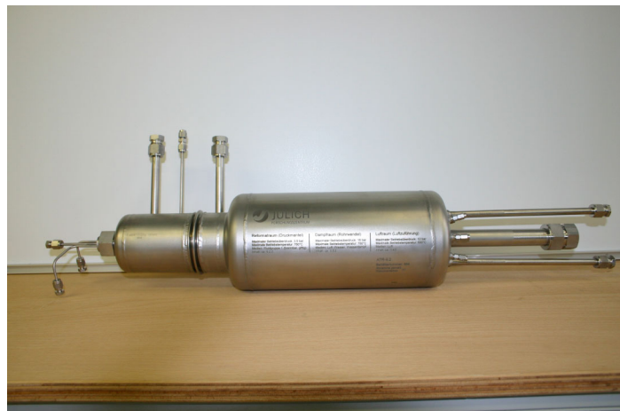
Figure 2: Autothermal reformer of the ninth generation (ATR 9.2) of Forschungszentrum Jülich
