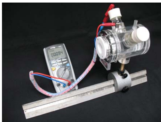
Picture 1: TriplePowerCell assembly which adopts a silicide cathode as light receiver and a transition metal anode and is filled with an electrolyte (e.g., water - sulfuric acid or a base or salts). The system is able to a) split water into hydrogen and oxygen under acidic conditions where the product gases can be separated by a membrane, and b) the system allows to collect additionally or separately electricity, and c) the TriplePowerCell allows to collect residual thermal energy by way of a heat exchanger.
