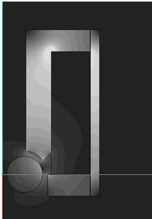
Figure 2: Model of the magnetic circuit of the RRV®. The qualitative distribution of the value of the magnetic field B was calculated and shown as grey levels. The lighter the grey level the stronger the magnetic field strength.
