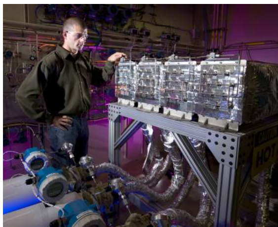
Figure 1: A full scale hydrogen storage system designed for automotive fuelling requirements.
