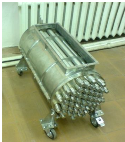
Figure 2: Tube-and-shell type hydrogen storage device, combined air and liquid cooling/ heating, 81 kg of AB_5 alloy.
