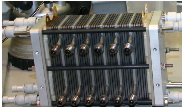
Figure 1: Liquid cooled HT-PEM-Stack with 28 cells by ZBT.
