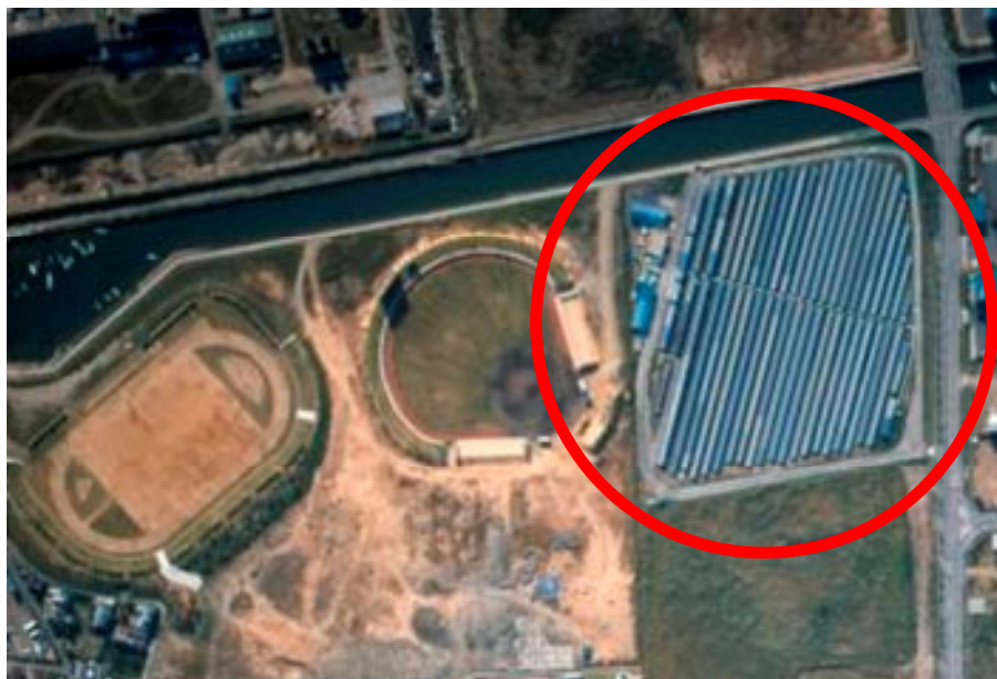
Figure 1: A solar system test facility of 1,000 kW with 22,000 solar panels.
