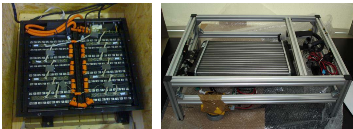
Figure 7: 80 cells BS and BS test cooling network.
