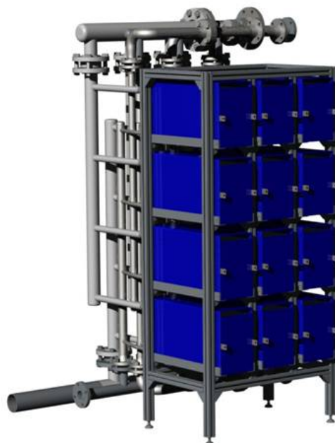
Figure 1: Module with 12 stacks, with 75 cells each and an effective cell area of 200 cm 2 .
