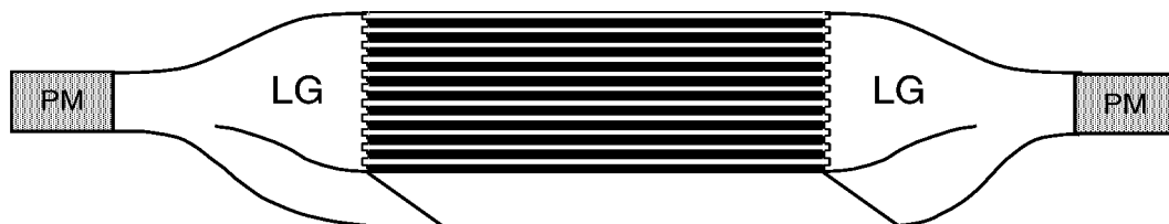
Figure 3.10: Scheme of a neutron detector module. 11 plastic scintillator plates (white layers) are interlayed by the same amount of lead sheets (dark layers). LG and PM denote light guides and photomultipliers, respectively.
