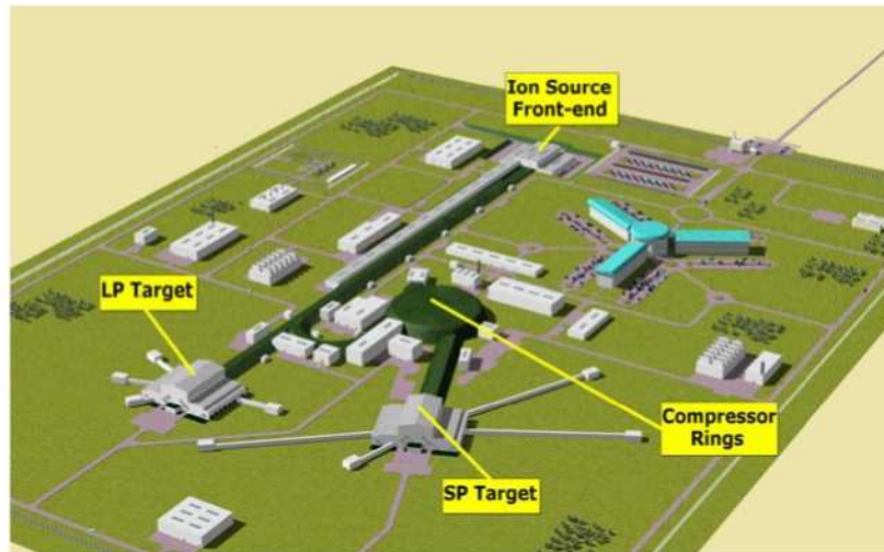
Figure 2.3: ESS - a possible layout: Artist's view of the ESS facility showing the ion source, the linac tunnel leading to the accumulator and compressor rings from where the beam is distributed to the short pulse target station. The long pulse target station with instruments is directly connected to the linac.
