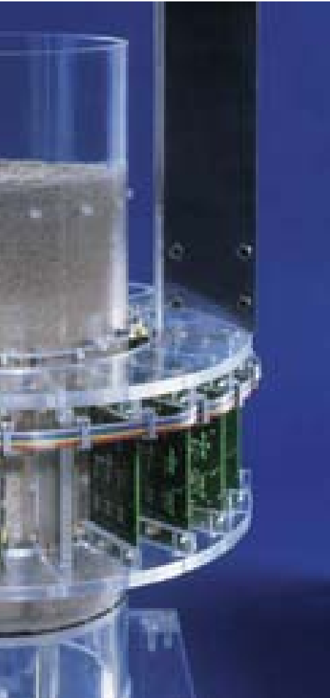
A ring of magnetic field sensors provides information on soil structure, moisture and transport paths for contaminants from deep within the soil.
