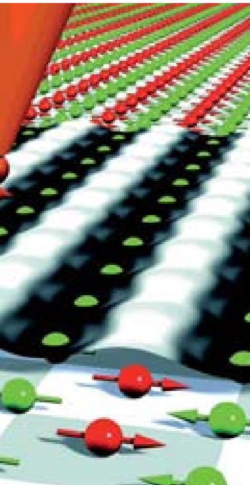
The magnetic tip of a spin-polarised scanning tunnelling microscope scans a magnetic layer in which the atomic spins are oriented in the opposite direction.
