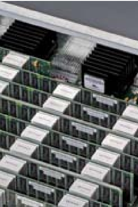
64 processors on 16 cards fill a drawer in the JUBL supercomputer. Supply and control chips are also needed.
