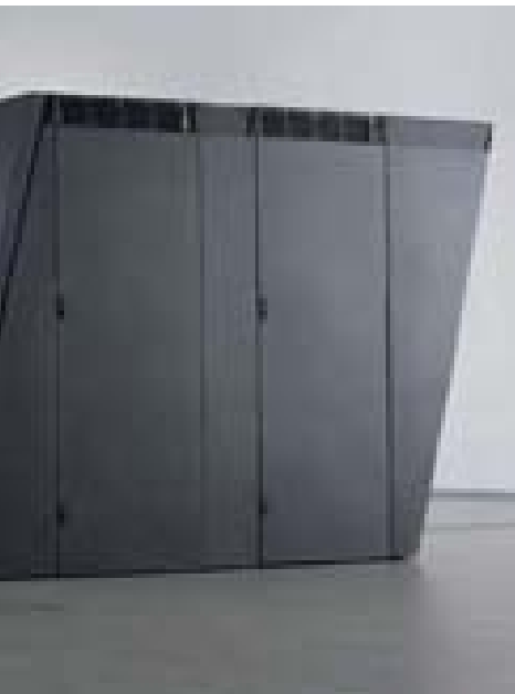
JUBL: a total of 16 384 processors operate in its four climate-controlled racks.
