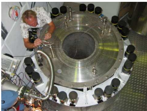
Fig. 1: The new magnet of the ATRAP collaboration with its 50 cm-bore.
