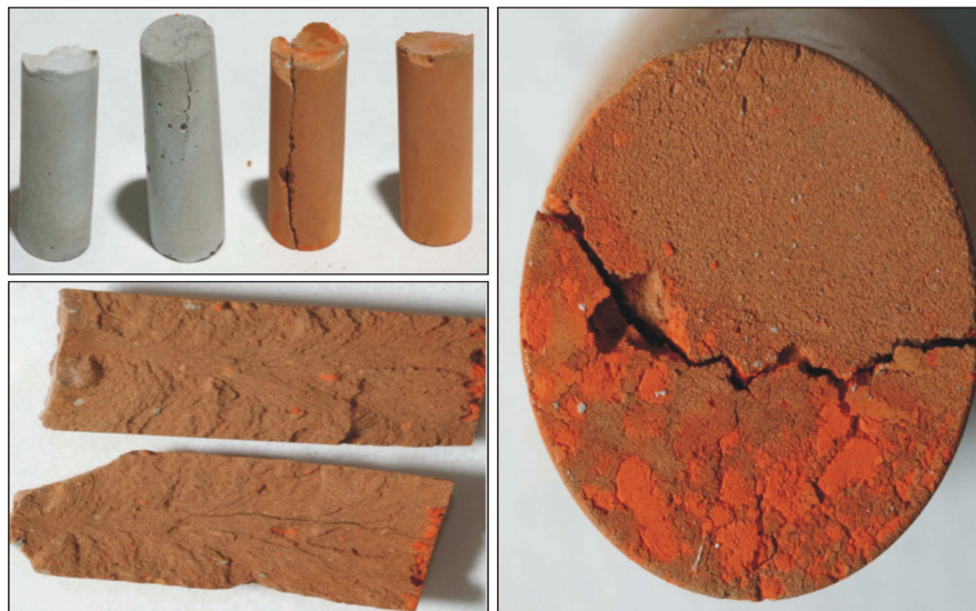
Figure 35: Concrete specimen containing mercury compounds
