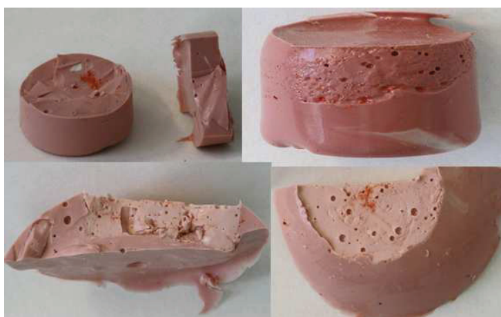
Figure 43: HgS/polysiloxane specimen - unlayered (top) and layered (bottom)
