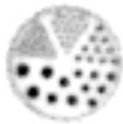
Figure 8. Central slice of a Micro Deluxe phantom (Data Spectrum Corp.) with an inner diameter of 4.5 cm and hollow channel diameters of 1.2, 1.6, 2.4, 3.2, 4.0 and 4.8 mm.
