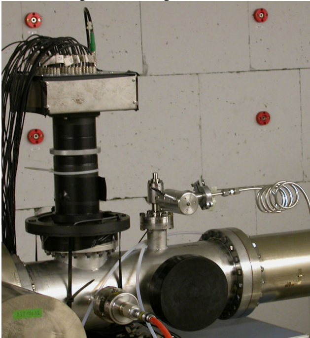
Fig. 1: The new SPM setup. Shown are the vacuum chamber, the piezo-electric leak valve with its nitrogen line and the light detection system consisting of the PMT and a lens.
