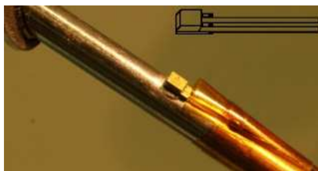
Fig. 3: Temperature diode soldered on a stainless steel target finger, superimposed is the mechanical layout of the diode.
